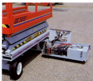
"Swing-out" drawers permit full access to all hydraulic and electric components for easy service and maintenance.
