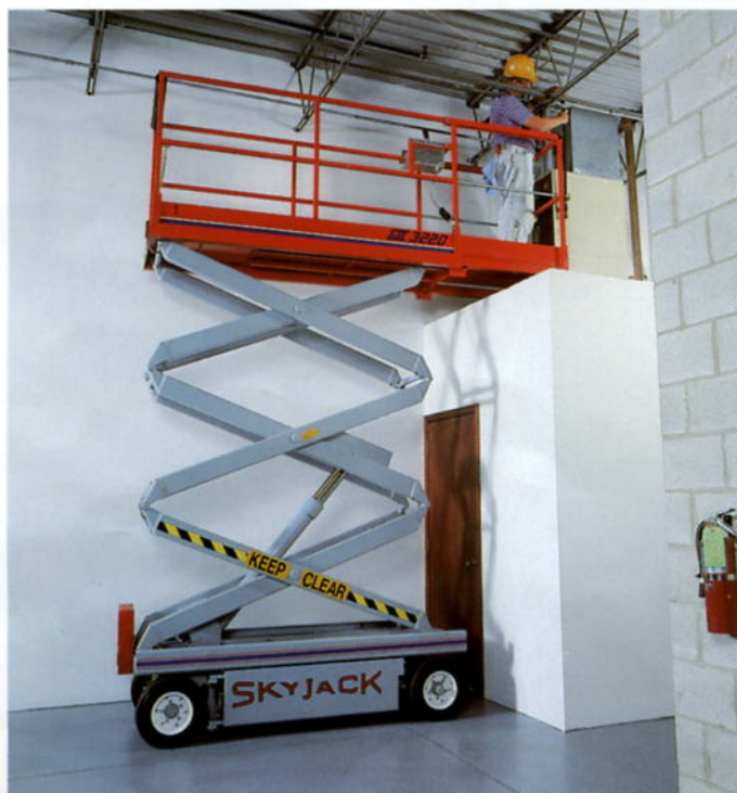
3' (0.91m) roll out deck extension provides larger work area and versatility.
