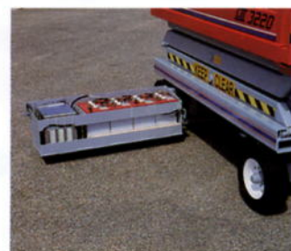
All batteries and charger are conveniently located in one tray for fast and easy maintenance checks.
