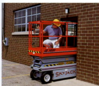
Narrow width allows SJII Model 3220 to pass through standard doorways and narrow aisles.
