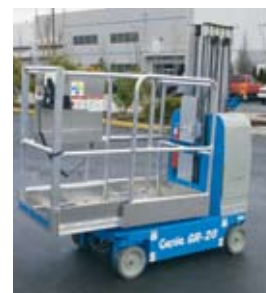
SLIDING MID-RAIL EXTENSION DECK PLATFORM 140 x 75 cm (55 x 29.5 in) Provides 51 cm (20 in) of horizontal outreach and a larger work area within the platform.
