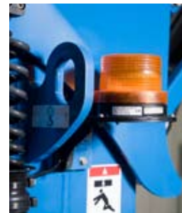
RUNABOUT™ WITH JIB Optional flashing beacons
