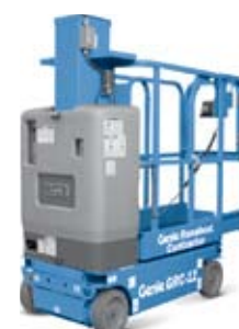
STEEL PLATFORM AND EXTENSION DECK WITH SWING GATE 140 x 75 cm (55 x 29.5 in) provides 44 cm (17.5 in) of horizontal outreach and allows up to two people in the platform.
