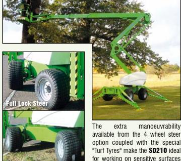
available from the 4 wheel steer option coupled with the special "Turf Tyres" make the SD210 ideal for working on sensitive surfaces such as grass.
