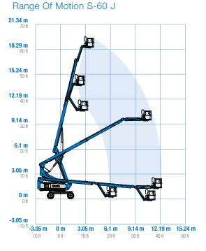
\* The metric equivalent of working height adds 2 m to platform height. U.S. adds 6 ft to platform height.
