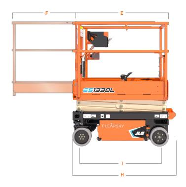
A. Platform Height (Lowered) 28-in / 0.7-m B. Platform Railing Height 43.3-in / 1.1-m C. Machine Height 71.7-in / 1.8-m Platform Width 24.4-in / .6-m E. Platform Length 49.2-in / 1.3-m
